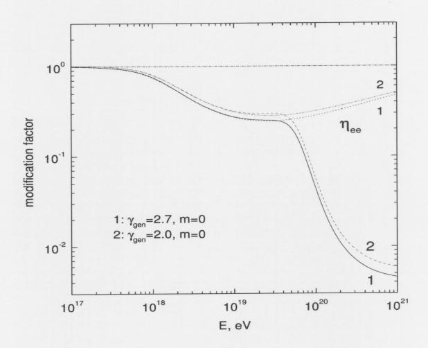
The dotted curve shows  $\eta_{ee}$ , when only adiabatic and pair-production energy losses are included. The solid and dashed curves include also the pion-production losses.
