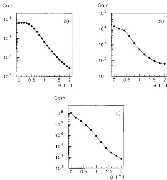
Fig. 1. Gain of the fine mesh phototubes as a function of the magnetic field strength parallel to the tube axis. (a) 1 in. tube,  $U = 2000$  V; (b) 1.5 in. tube,  $U = 2000$  V; (c) 2 in. tube,  $U = 2500$  V.
