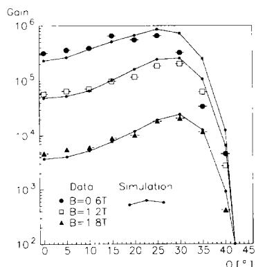
Fig. 8. Measured and simulated (full line) gain of an 1 in. phototube as a function of the angle  $\theta$  between the phototube axis and the magnetic field.
