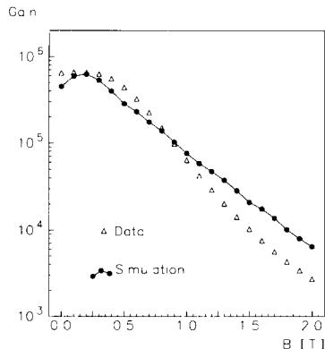
Fig. 7. Comparison of measured and simulated gain of an 1 in. phototube as a function of the magnetic field  $B$ . The curves are normalized to each other at 0.2 T.
