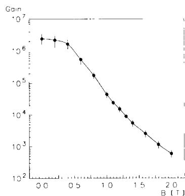
Fig. 2. Average gain of four 1 in. phototubes ( $U = 2000$  V) as a function of the magnetic field  $B$ . The length of the error bars indicates the variance of the sample
