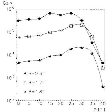
Fig. 3. Gain of the 1 in. phototube as a function of the angle  $\theta$  between the tube axis and the direction of the magnetic field for three different field strengths  $B$ . The full lines are included to guide the eye.
