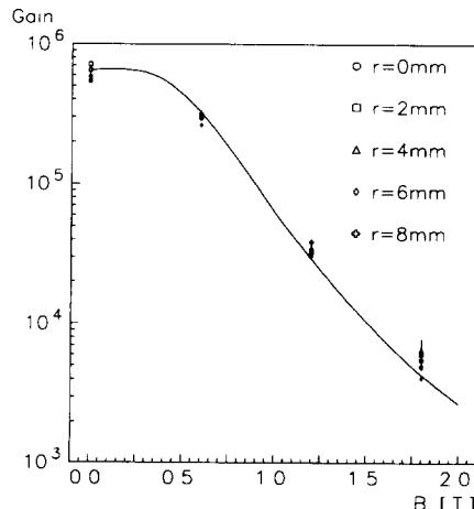
Fig. 4. Gain of the 1 in. phototube as a function of the field strength  $B$  for different impact points of the photons on the cathode.
