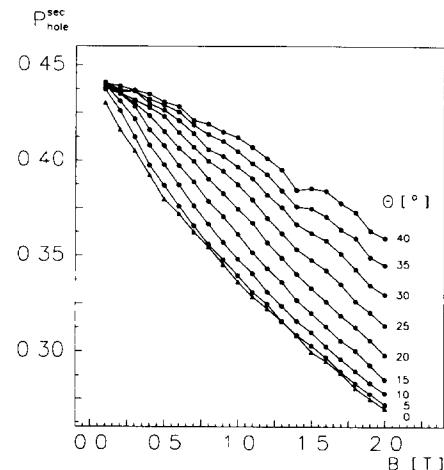
Fig. 6. Probability  $P_{\text{hole}}^{\text{sec}}$  of a secondary electron to pass a hole of the mesh for different angles between the phototube axis and the magnetic field. The lines are shown to guide the eye.
