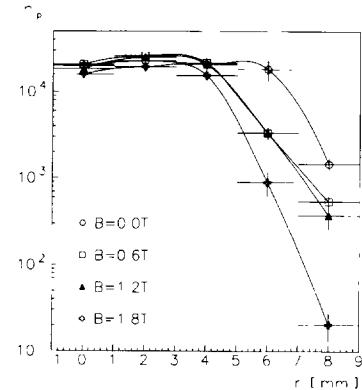
Fig. 5. Number of photoelectrons for the 1 in. phototube as a function of distance of the impact point from the phototube axis for different field strength  $B$ .
