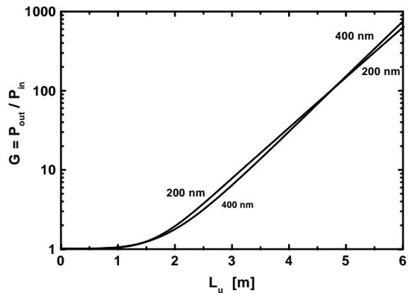
Fig. 3. Power gain,  $G = P_{out}/P_{in}$  versus undulator length for the FEL amplifier operating at 200 and 400 nm wavelength (radiation beam size at the undulator entrance  $w$  is equal to 400 and 800  $\mu\text{m}$ , respectively).
