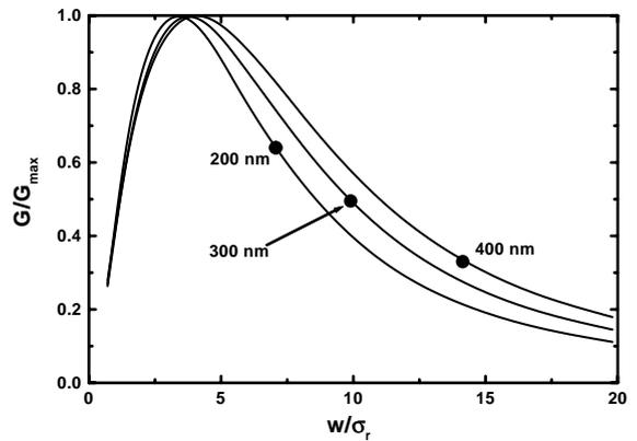
Fig. 2. Power gain in the linear regime versus spot size of the seeding radiation beam (the rms transverse size of the electron beam is  $\sigma_r = 55 \mu\text{m}$ ).
