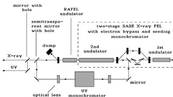
Fig. 1. Schematic layout of the pump-probe facility combining UV regenerative FEL amplifier and soft X-ray FEL at TTF.
