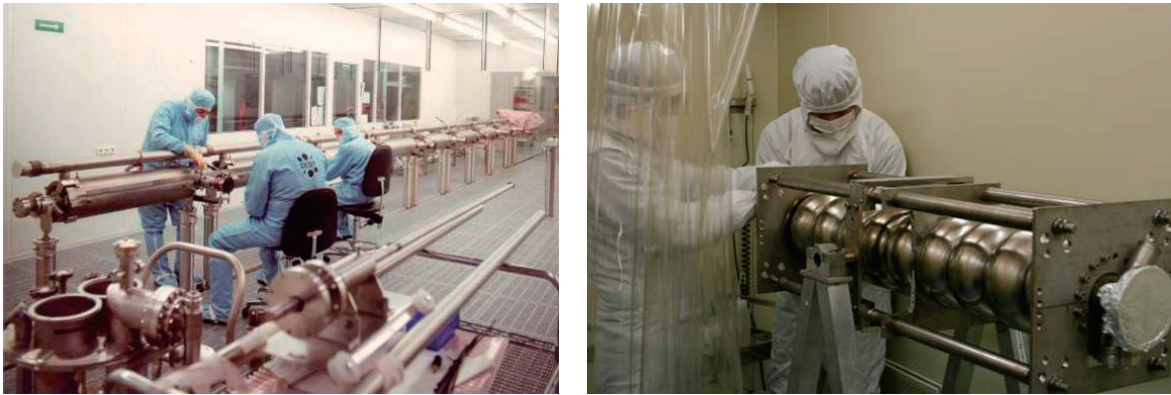
FIGURE 2.4. Clean room environments are mandatory. Left: the assembly of eight nine-cell TESLA cavities into a cryomodule string at DESY. Right: an ICHIRO nine-cell cavity is prepared for initial tests at the Superconducting RF Test Facility (STF) at KEK.
