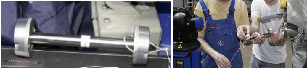
Figure 30. The “mouse” survey tool, used to measure the position of the middle of the beam pipe along the magnet.
