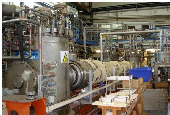
Figure 26. Test bench with the HERA dipole used for the ALPS-I experiment. It is located in hall 55 and will be used to test all dipoles foreseen for ALPS-IIc.
