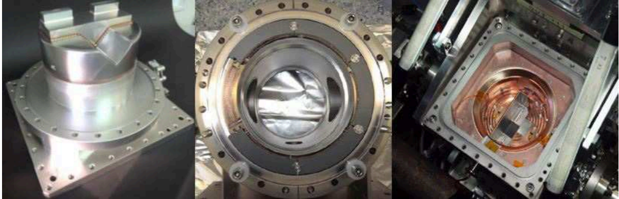
Fig. 9.3: Three of the main modifications implemented to minimise the effect of RF. From left to right: the RP filler with the copper contacts for proper grounding, the ferrites distributed as a ring on the flange of the station and the HDS (heat distribution system) in copper with the temperature probes attached to it.
