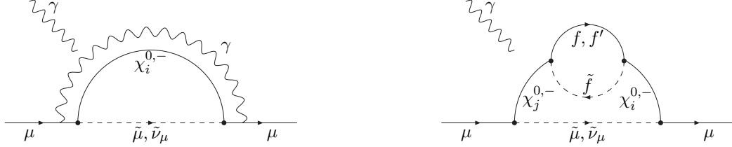
Figure 2: Sample two-loop diagrams corresponding to SUSY one-loop diagrams with additional photon loop (left), or with fermion/sfermion-loop insertion (right). The external photon can couple to each charged particle.
