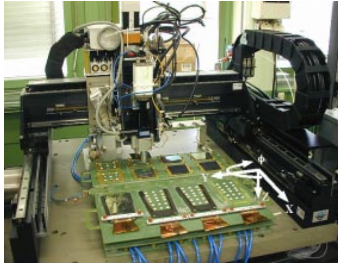
Figure 25: Photograph of a gantry robot as used in the construction of silicon detector modules for the current CMS tracker [29].
