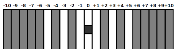
Figure 7: Default illumination pattern for images at the equator [11]. Stripes are numbered from left to right, starting with -10 and ending with +10. Grey stripes are switched off, white stripes are switched on. The dark square in the center indicates the opening for the camera.
