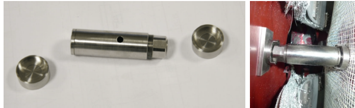
Figure 10: Outer pressure prop parts (left) and prop inserted into the cryostat (right).
