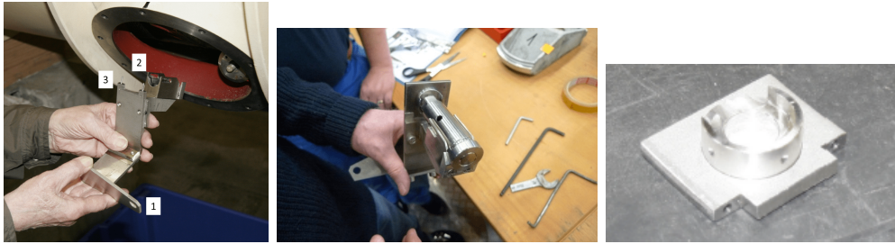
Figure 18: Tool for proper placing of the outer pressure props. Left: 1: Plate to fasten the tool to the flange of the vacuum vessel, 2: Cradle to hold the pressure prop, 3: Pins to connect to the outer pressure plate. Middle: Complete prop in the assembly tool. Right: Outer pressure plate with support cup.
