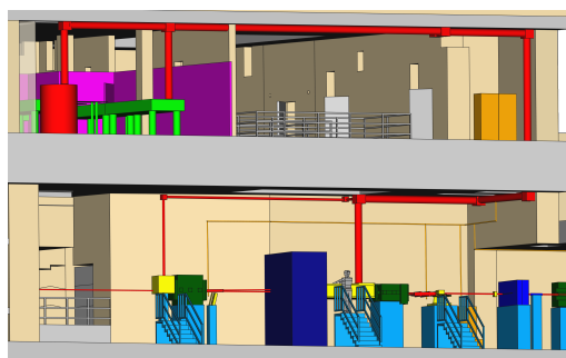
Figure 8.4. CAD drawing of the XS1 access shaft building, including the LUXE experiment, zoomed on the laser transport pipe from the clean-room to the interaction point. The ICS setup is also shown. The building is shown in beige and grey, while the different experimental elements are shown coloured.
