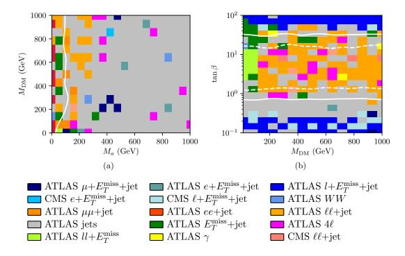
Figure 5: Sensitivity scans in (a)  $M_{\rm DM}$  vs  $M_a$  and (b)  $\tan \beta$  vs  $M_{\rm DM}$ ; the colours indicate the most sensitive set of measurements. The 95% (68%) excluded contours are indicated by solid (dashed) white lines; note that the whole plane in  $M_{\rm DM}$  vs  $M_a$  is excluded at 68% confidence level. All other parameters are as given in Table 1.
