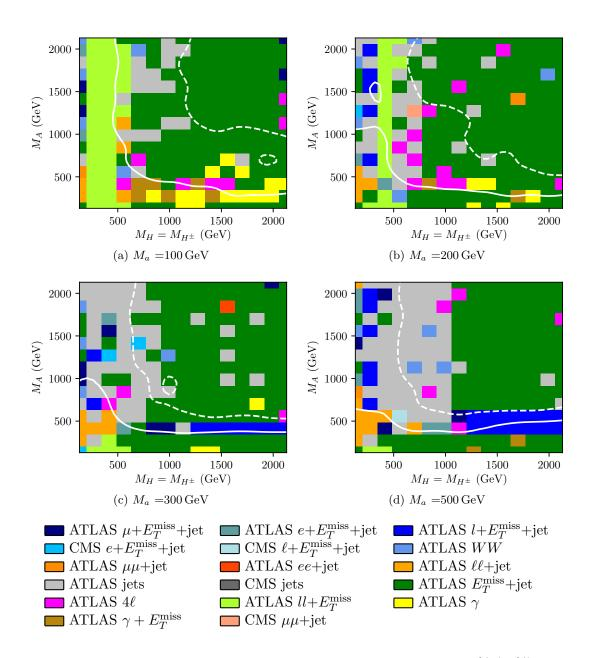
Figure 3: Sensitivity scan in  $M_A$  vs  $M_H = M_{H^{\pm}}$  for different  $M_a$ . The 95% (68%) excluded contours are indicated by solid (dashed) white lines; the colours indicate the most sensitive set of measurements. All other parameters are as given in Table 1.
