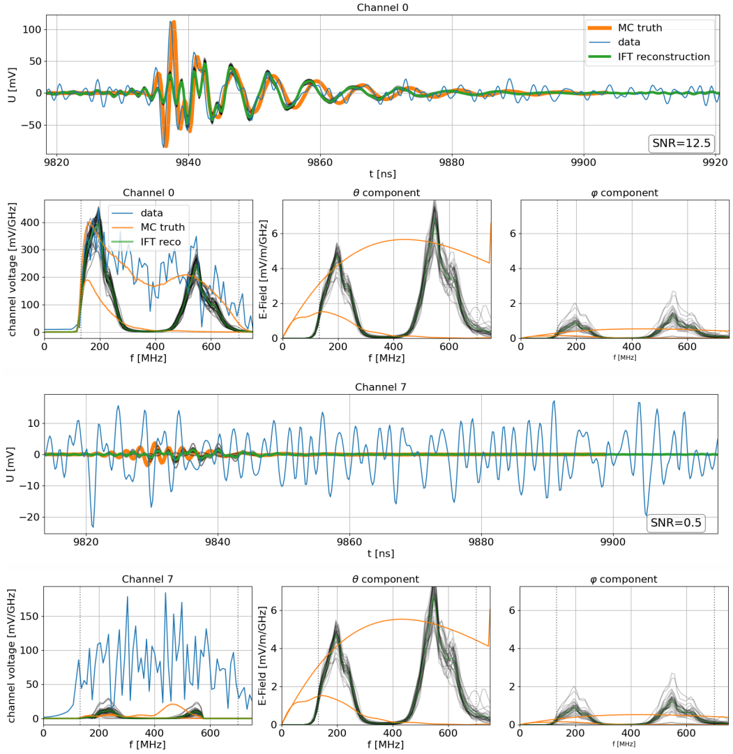
Figure 17. Results of a failed electric field reconstruction of an event detected by an RNO-G station. Shown are one of the Vpol (top) and one of the Hpol (bottom) channels. 1st and 3rd row: Waveform of the data (blue), the actual signal (orange) and the reconstruction (green). 2nd and 4th row: Spectrum of the channel voltage (left) and the \vec{e}_\theta (center) and \vec{e}_\phi (right) component of the electric field. The thin gray lines are the samples used for uncertainty estimation.
