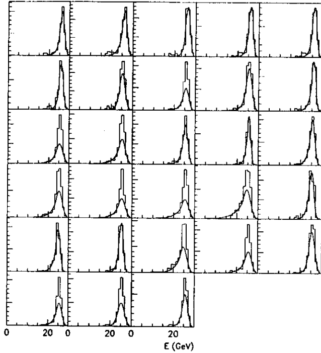
Figure 6.10: The electron energy spectra in the correction bins, for the Monte Carlo KP sample. The histograms from left to right and top to bottom follow the numbering scheme of fig. 6.8, with the top left and bottom right histograms corresponding to bins 1 and 28, respectively.
