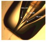
Figure 3. Water flowing through a 50micron inner diameter tube can be seen to form a tapering jet as the liquid is accelerated by a coaxially flowing helium gas sheath.
