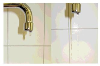
Figure 1. Dripping and jetting from a water faucet.
