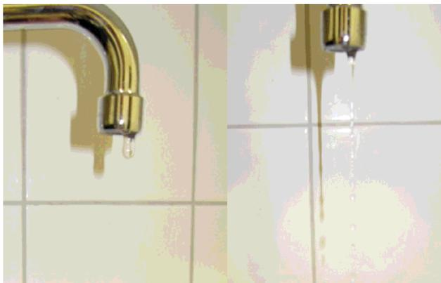
Figure 1. Dripping and jetting from a water faucet.
