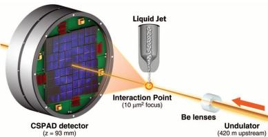
**Fig. 1.** Experimental geometry for SFX at the CXI instrument. Single-pulse diffraction patterns from single crystals flowing in a liquid jet are recorded on a CSPAD at the 120-Hz repetition rate of LCLS. Each pulse was focused at the interaction point by using 9.4-keV x-rays. The sample-to-detector distance (z) was 93 mm.
