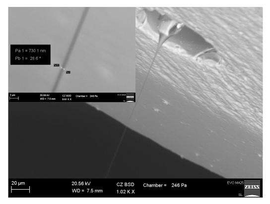
**Figure 5.3:** Environmental Scanning Electron micrograph of a tip of gas dynamic virtual nozzle in operation. Inset in the upper right corner presents measurement of the jet diameter ( $D=730 \mathrm{nm}$ ) measured approximately 40  $\mu \mathrm{m}$  from the nozzle tip. Flow rate of that nozzle has been measured using Sensirion flow sensor, at that liquid pressure conditions (40psi) it was 1.2  $\mu \mathrm{l}/\mathrm{min}$ .
