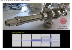
Figure 6. An aerodynamic lens currently in use at LCLS and FLASH. Figure is courtesy of Janos Hajdu.
