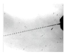
Figure 2. A water jet driven to breakup into 10micron drops by triggering at 200kHz.
