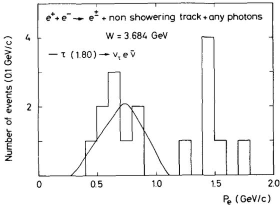
Fig. 1. Raw electron momentum distribution observed at 3.684 GeV. The events have one identified electron, one nonshowering particle, and any number of photons.
