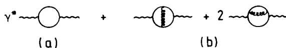
Fig. 12.1 Gluonic QCD corrections (b) to the zeroth order e^+e^- annihilation cross section (a).
