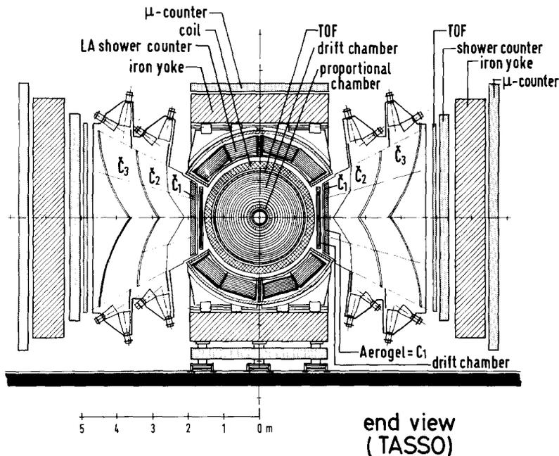
Fig. 1. View of the TASSO detector along the beam line.
