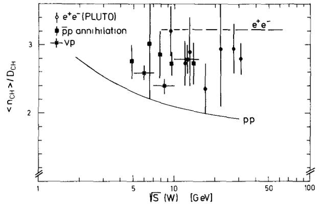
Fig. 3. Energy dependence of the ratio  $\langle n_{ch} \rangle / D_{ch}$ . For comparison data from pp [13],  $\bar{p}p$  annihilations [14] and  $\nu p$  [15] interactions are also shown. The dashed line indicates the QCD prediction [4] for  $e^+e^-$ .
