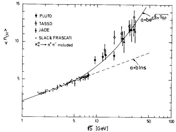
Fig. 1. Energy dependence of the average charged multiplicity for  $e^+e^-$  annihilations. Data below 7 GeV are from Frascati and SLAC [10] and at higher energies from DORIS [7] and PETRA [11]. Only for a few Frascati and SLAC points errors are marked. JADE points are the observed multiplicities. Both statistical and systematic errors are included.  $K_s^0 \rightarrow \pi^+\pi^-$  decays are included.
