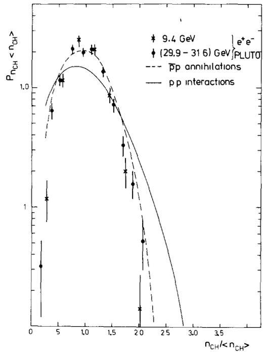
Fig. 4. KNO plot for  $e^+e^-$  annihilation (PLUTO data at 9.4 and 30.7 GeV). The dashed curve is the fit to  $\bar{p}p$  annihilations [16] and the full curve is for high energy pp collisions [13].
