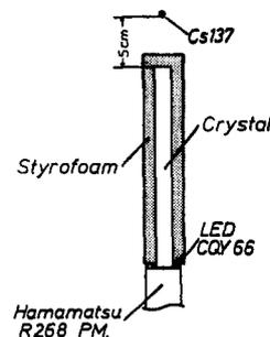
Fig. 2. Arrangement of crystal and photomultiplier.
