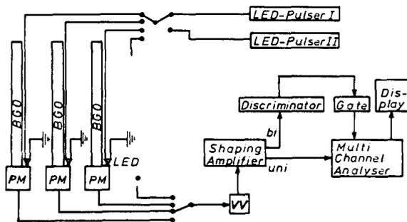
Fig. 1. Readout setup for measuring pulse heights from BGO and CsI scintillating crystals.
