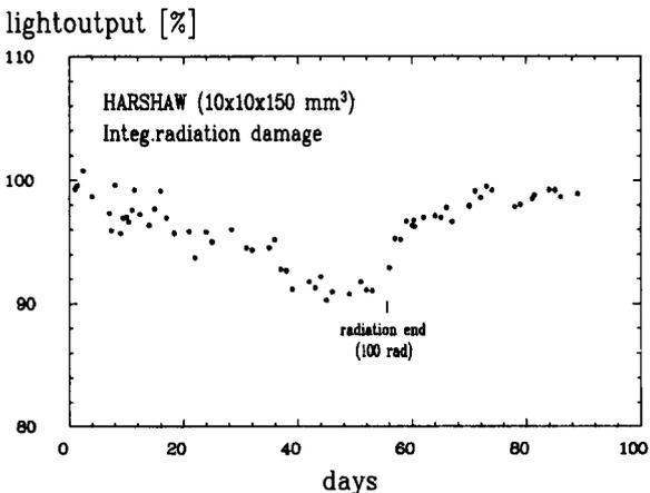
Fig. 9. Pulse height history of a 15 cm long BGO crystal exposed to background radiation on the PETRA beam pipe for 53 d.
