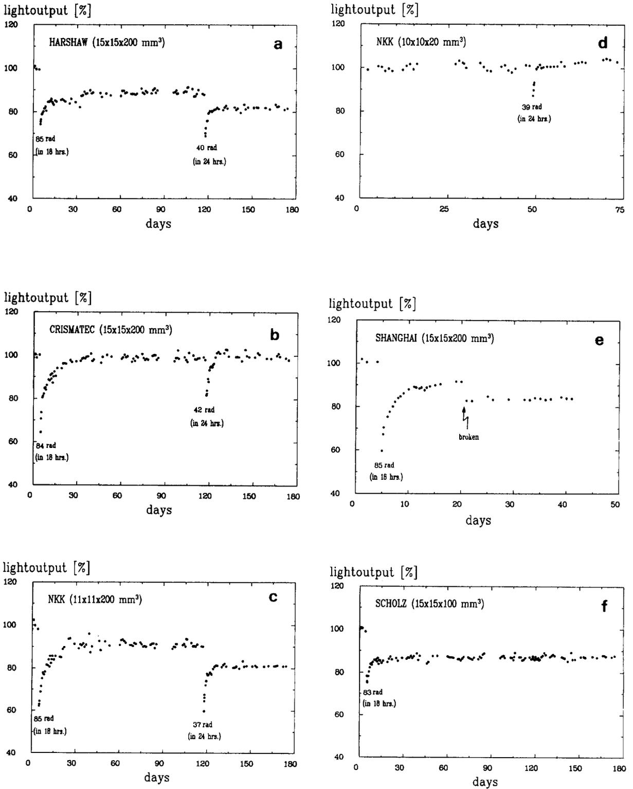
Fig. 4. (a)–(f) Pulse height history of various BGO crystals which were subject to short term radiation exposures. Plotted is the light output normalized to the light output measured before the first exposure. The radiation doses refer to the readings from the TLDs mounted on the front face of the crystal.
