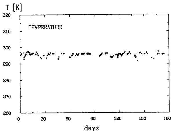
Fig. 3. Temperature history of the crystals used for short term radiation exposures to a  $^{137}\text{Cs}$   $\gamma$ -ray source.
