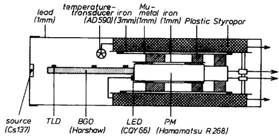
Fig. 7. Details of the BGO-box exposed to background radiation on the PETRA beampipe at the position shown in fig. 6.
