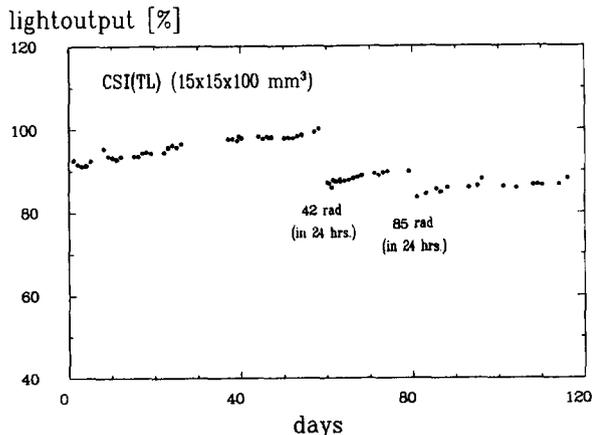
Fig. 5. Pulse height history of a CsI(Tl) crystal before and after two radiation exposures to a <sup>137</sup>Cs  $\gamma$ -ray source.
