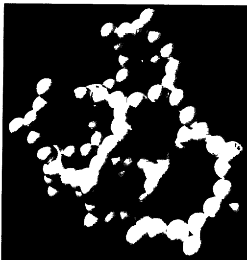
Fig. 4. Model of the structure of aerogel constructed according to Heesch and Laves [10]. In reality the particles have a diameter of about 40 nm and consist of clusters of silica colloides of about 4 nm in diameter. The particles are regularly packed with a coordination number of 3.
