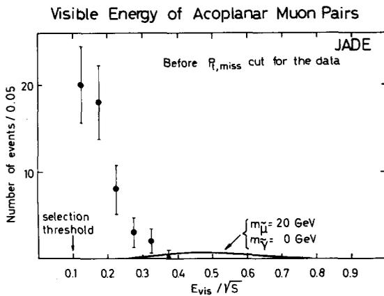
Fig. 3. The visible energy distribution of the acoplanar muon pair before the cut on the missing transverse momentum. The curve is an expected distribution for  $M_\mu = 20.0 \text{ GeV}/c^2$  and  $M_\gamma = 0 \text{ GeV}/c^2$ .
