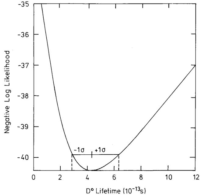
**Fig. 3.** The negative logarithm of the likelihood function for the fifteen reconstructed proper decay times. The one standard deviation errors are indicated
