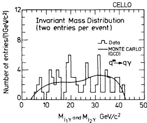
Fig. 2. Jet–photon invariant mass distribution from events with two-jets plus an isolated photon.
