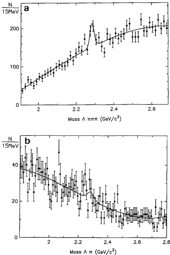
Fig. 3. Invariant mass distribution, with  $x_p > 0.5$ , for (a)  $\Lambda_c^+ \rightarrow \Lambda \pi^+ \pi^- \pi^+$  and (b)  $\Lambda_c^+ \rightarrow \Lambda \pi^+$  combinations. The solid line is the best fit using a gaussian for the  $\Lambda_c^+$  and a polynomial background.
