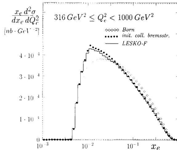
Fig. 3. Distributions of differential cross section  $x_e d^2\sigma/dx_e dQ_e^2$  obtained from LESKO-F (solid line) and from non-Monte Carlo calculations: in the Born approximation ( $\diamond\diamond\diamond$ ) and in the collinear bremsstrahlung approximation ( $\bullet\bullet\bullet$ ) (see section 5).
