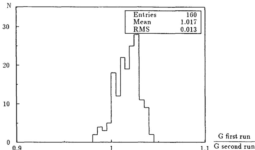
Fig. 15. Test of reproducibility using the cobalt source as an absolute reference standard. Scans were taken 11/2 months apart and the profiles for each HAC1 tower were integrated.
