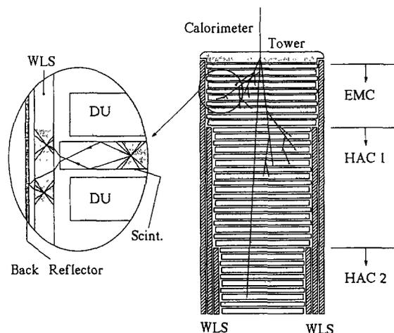
Fig. 1. Schematic representation of a uranium/scintillator stack read out by wavelength shifter light guides (not to scale).
