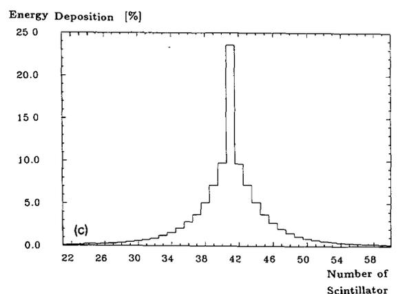
Fig. 10. Energy deposition patterns as determined by the EGS4 Monte Carlo. (a) First interaction points of photons in a scintillator tile. (b) Projection of the plot in (a) indicating that the mean depth of penetration of the cobalt photons is 15 mm. (c) Energy deposition as a function of layer number in the calorimeter stack.
