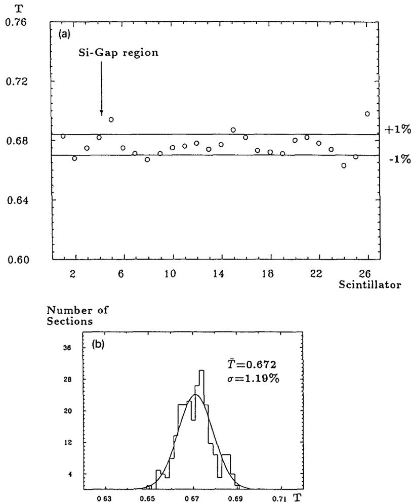
Fig. 11. (a) Transmission  $T$  vs scintillator number in a typical EMC tower indicating that the attenuation length in the scintillator tiles is uniform to within 1%. (b) Distribution of average values  $\bar{T}$  from all HAC1 sections in 15 FCAL modules.
