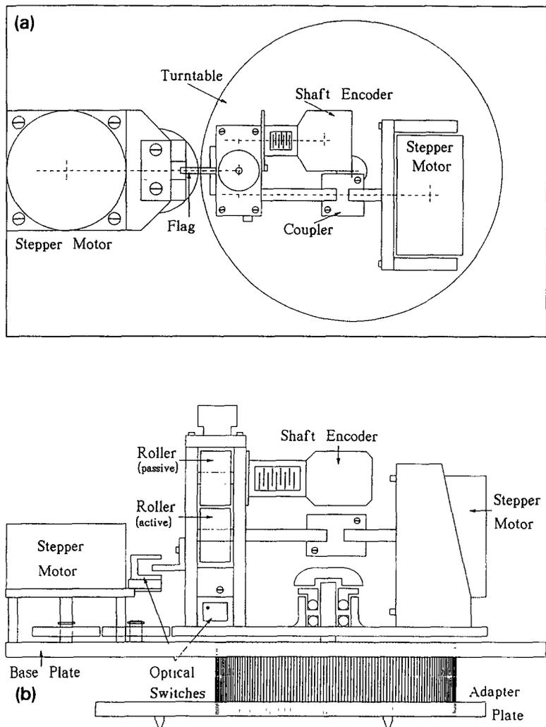
Fig. 5. The source driver, (a) top view, (b) side view.
