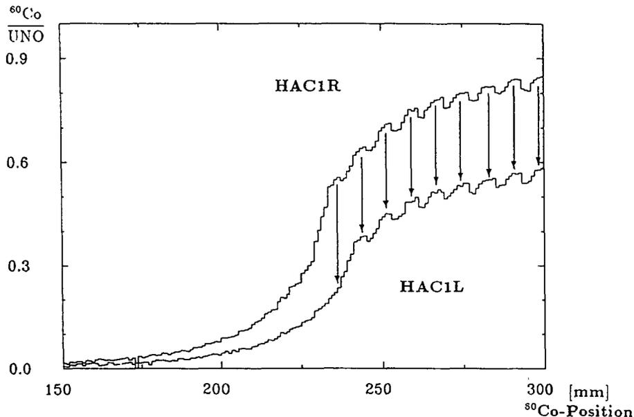
Fig. 13. Scan indicating the misalignment of a WLS cassette of the left side such that the first scintillator of the HAC1 stack is seen by the right WLS, but not by the left one.
