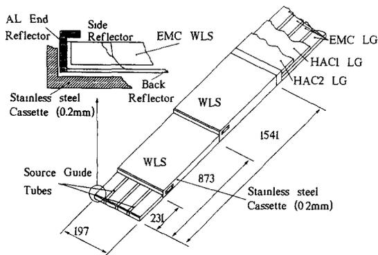
Fig. 4. Detail of how the guide tubes are incorporated into the light guide assemblies.
