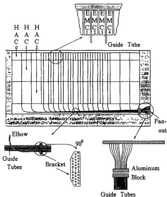
Fig. 3. The tube system for guiding the cobalt source inside the calorimeter modules.
