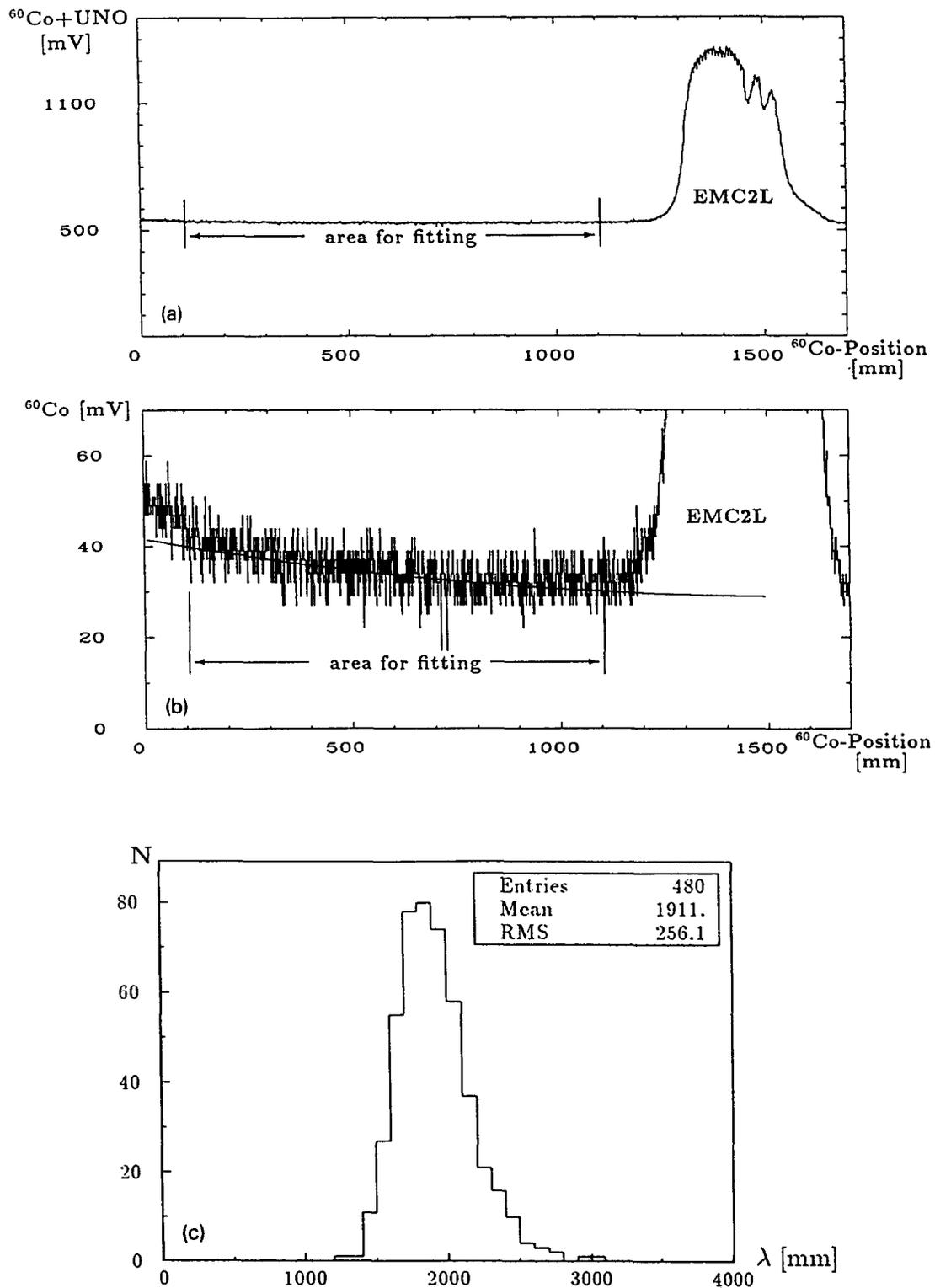
Fig. 12. (a) Current vs source position for a typical EMC light guide. (b) As in part (a) but with UNO signal subtracted and an exponential fit. (c) Distribution of attenuation lengths in all EMC light guides in all inside scanned FCAL modules.
