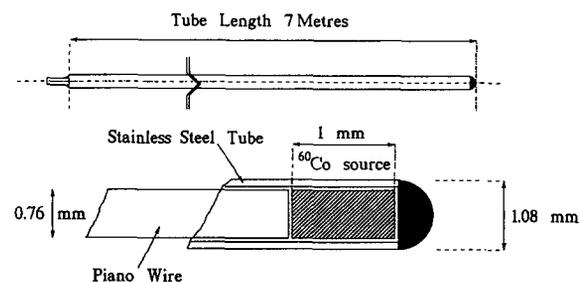
Fig. 6. The source assembly. Active cobalt is encapsulated within a stainless steel tube with a closed end. It is held in with a flexible filler wire.
