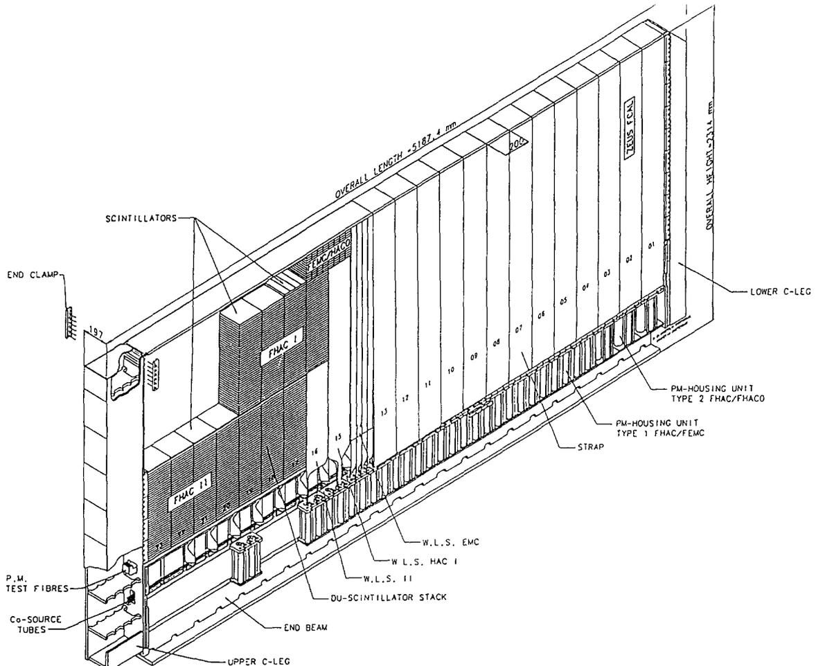
Fig. 2. Isometric view of a the largest forward calorimeter (FCAL) module, illustrating the tower structure and some construction features.
