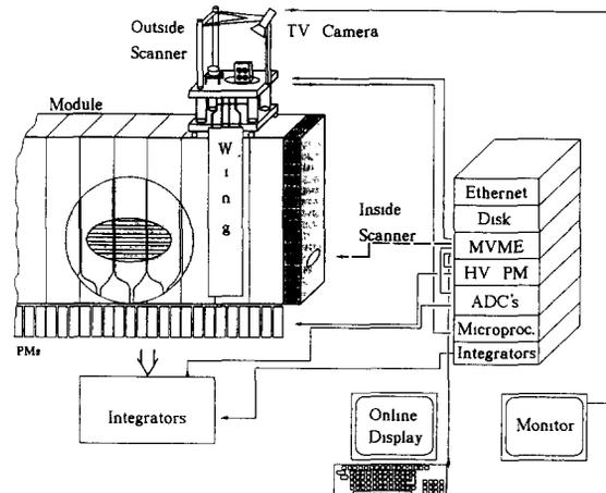
Fig. 7. The "outside" scanner used for most of the data presented in this paper.
