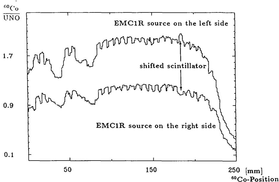
Fig. 14. Scan indicating a shifted scintillator tile. The particular layer shows up as a spike on one side of the tower and a dip on the other.
