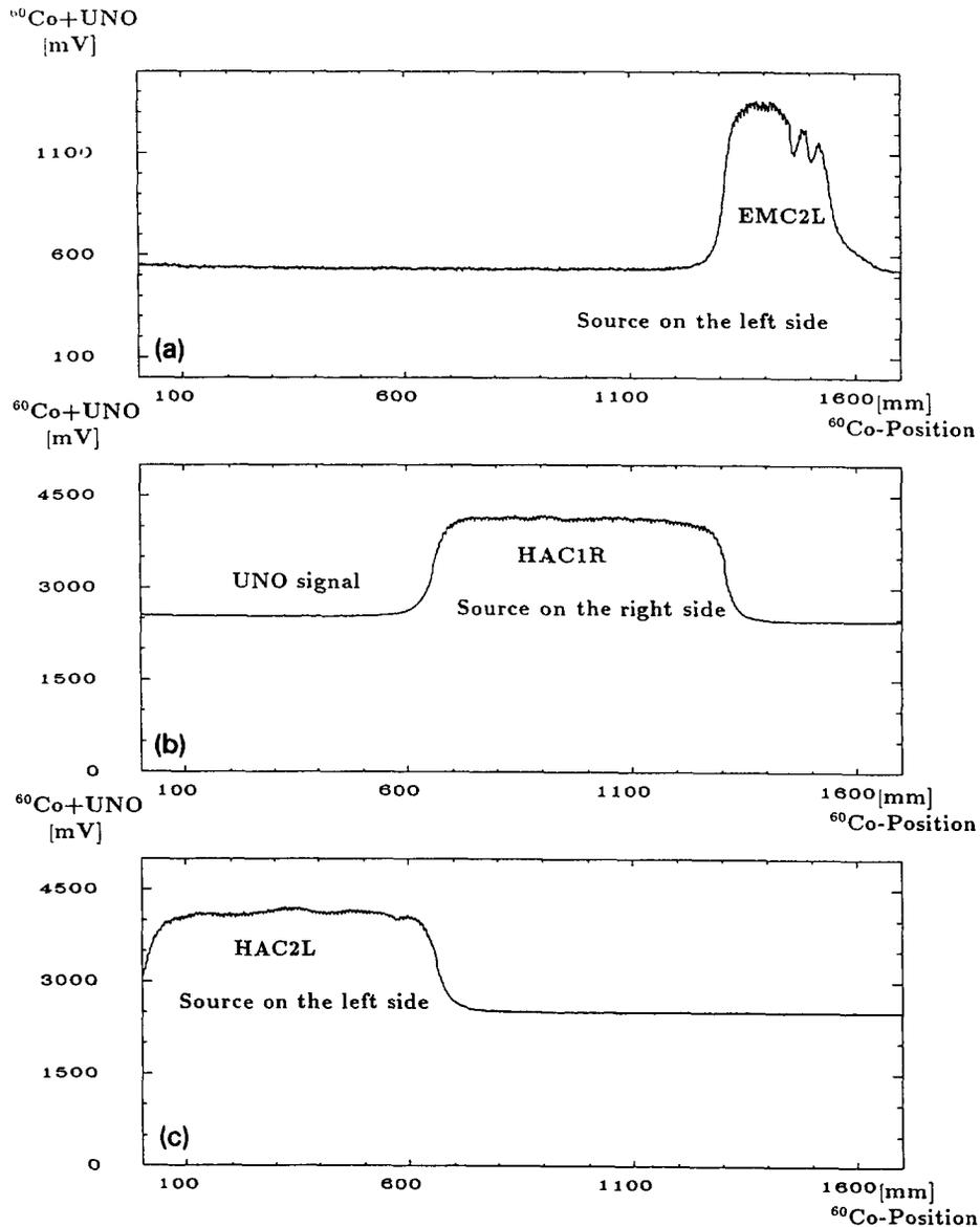
Fig. 8. Typical data from a source scan for (a) EMC, (b) HAC1 and (c) HAC2 sections of a tower. Note the fine structure which results from the layer construction of the calorimeter. The background is due to the uranium activity (UNO). EMC2L for example indicates the read out of the left PMT.
