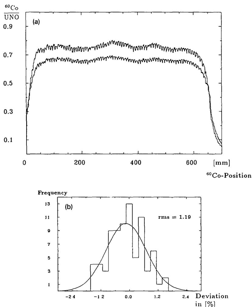
Fig. 9. Comparison of two different scans done to test reproducibility. (a) Data from a typical tower. The upper curve was taken using the inside scanner at CERN and the lower curve was taken using the outside scanner, months later at DESY. (b) The ratio of the curves plotted in (a) is calculated for identical source positions. (b) presents the frequency distribution of the derivation of this ratio ( $S_L/S_R - 1$ ) from the mean value.
