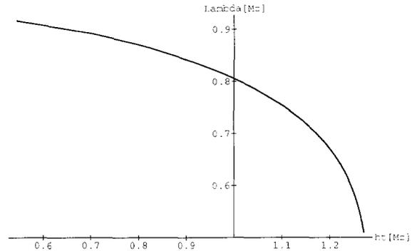
Fig. 1. Values of  $\lambda(M_Z)$  for variable  $h_t(M_Z)$  calculated with the RGE of eq. (29), (30) with the saturation condition  $\lambda^2(A)/4\pi = 1$  and  $A = 10^{16}$  GeV.
