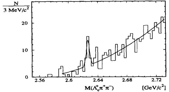
Fig. 4. The invariant mass distribution for  $\Lambda_c^+ \pi^+ \pi^-$  combinations satisfying both  $|M(\Lambda_c^+ \pi^+) - M(\Sigma_c^{++})| > 5.1 \text{ MeV}/c^2$  and  $|M(\Lambda_c^+ \pi^-) - M(\Sigma_c^0)| > 5.1 \text{ MeV}/c^2$ . The solid curve represents the fit described in the text.
