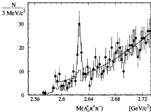
Fig. 1. Invariant mass distribution for all accepted  $\Lambda_c^+\pi^+\pi^-$  combinations. The solid histogram results from using the  $\Lambda_c^+$  sidebands.
