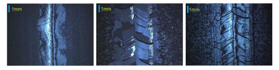
Figure 3: Equatorial welding seam of cell 1 in Z137: before EP (left), after main-EP (center) and after final-EP (right)
