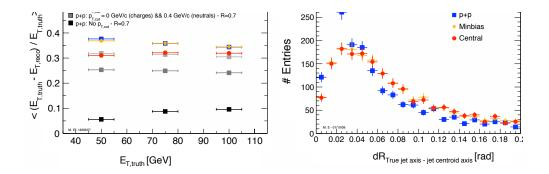
Fig. 4: <u>Left</u>: jet reconstruction efficiency as a function of  $E_{T,truth}$  for the cases quoted in the top left legend of the figure. <u>Right</u>: distance in  $\eta$ - $\phi$  space between the directions of the reconstructed jet axis and the true one in p + p (squares), Pb + Pb Minbias (stars) and Pb + Pb Central (circles) collisions.
