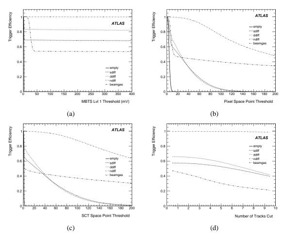
Fig. 3: The trigger efficiency for: MBTS\_2 as a function of the counter threshold (a), Pixel space point as a function of the number of Pixel space points required (b), SCT space point as a function of the number of SCT space points required (c), and track trigger as a function of the required number of reconstructed tracks (d).
