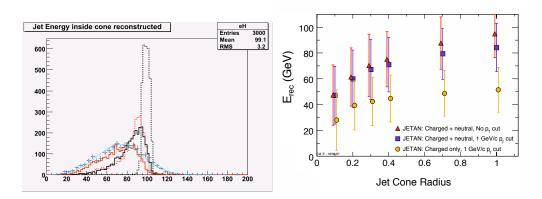
Fig. 1: <u>Left</u>: cone energy of 100 GeV jets reconstructed with PYCELL with R=1 (dark dashed line), with the ALICE cone finder with detector inefficiencies and acceptance included in the simulation with R=1 (red dashed), without detector effects but R=0.4 (dark full), with both effects (red full). The markers shows the result from a full simulation. <u>Right</u>: cone energy of  $100 \pm 5 \text{ GeV}$  fully simulated jets vs R for the three cases described in the text.
