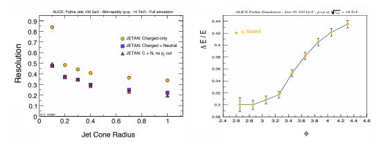
Fig. 2: <u>Left</u>: jet energy resolution of 100 GeV jets from a full ALICE simulation vs R for the three cases described in the text. Right: jet energy resolution as a function of the accepted  $\phi$  window of the center of the jet reconstructed.
