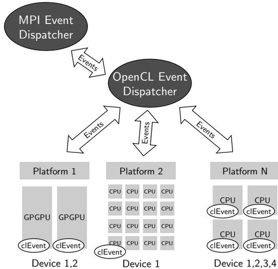
Figure 2: `OpenCL` dispatcher: the events are dispatched to different device queues. The different kernels to be processed are run asynchronously. The synchronization is performed thanks to `OpenCL events`
