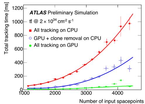
Figure 5: Track formation and clone removal show a 12x speed-up on NVIDIA C2050 GPU vs single-threaded Intel E5620 CPU. [8]
