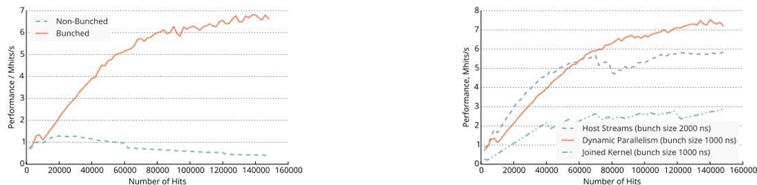
Figure 4: Performance for different optimization aspects of the Triplet Finder. Shown: Time needed to process a given number of hits, in million hits processed per seconds. *Left*: Comparison of Triplet Finder performance with and without bunching wrapper (optimal bunch size (1000 ns), dynamic parallelism approach). *Right*: Comparison of performance of different kernel launch strategies, invoked with respective ideal bunch sizes in bunching wrapper.
