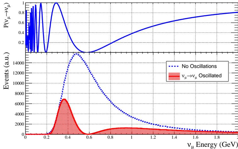
Figure 1: Effect of neutrino oscillation on a mock neutrino energy spectrum. Top plot shows the  $\nu_\mu$  survival probability and the bottom plot shows the mock energy spectrum with and without the survival probability applied.
