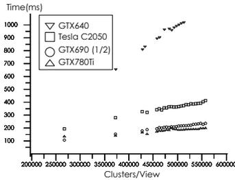
Figure 6: Absolute time (ms) for cluster correction and alignment. For GTX690, only one GPU is considered.
