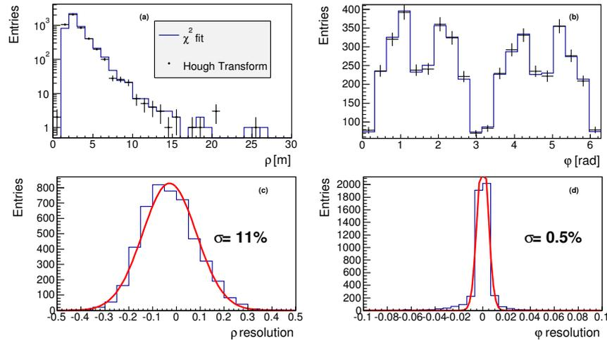
Figure 1: Hough Transform algorithm compared to  $\chi^2$  fit. (a)  $\rho$  distribution; (b)  $\varphi$  distribution; (c)  $\rho$  resolution; (d)  $\varphi$  resolution.
