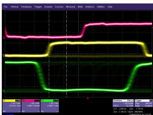
Figure 3: Deterministic latency of NaNet<sup>3</sup> SerDes: phase alignment of the transmitting (upper) and receiving (central) clocks.
