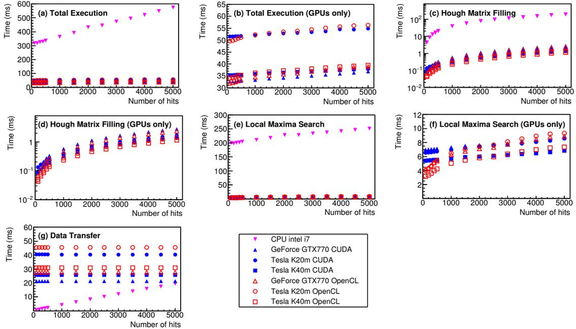
Figure 3: Execution timing as a function of the number of analysed hits. (a) Total execution time for all devices; (b) Total execution time for GPU devices only; (c)  $M_H$  filling time for all devices; (d)  $M_H$  filling timing for GPU devices only; (e) local maxima search timing for all devices; (f) local maxima search timing for GPU devices only; (g) device-to-host transfer time (GPUS) and I/O time (CPU).
