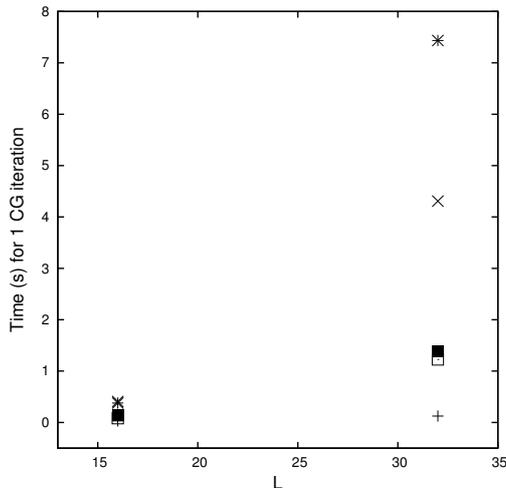
Figure 1: Weak scaling using lattice volumes  $V = L^4 = 16^4$  and  $32^4$  with 1 and 16 Tesla S1070 GPUs, respectively. The data correspond to the CG algorithm without preconditioning (+), with preconditioning **iii** (x), **iv** (\*), **iii** in single precision (□) and **iv** in single precision (■).
