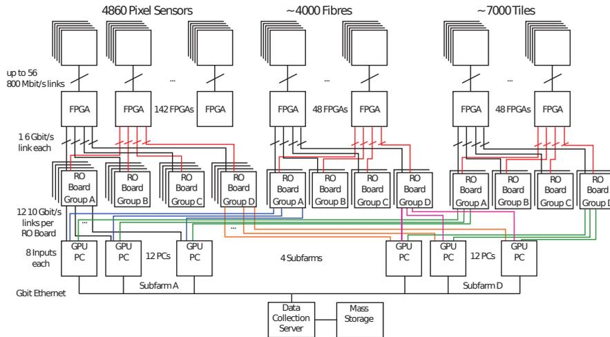
Figure 3: Readout scheme of the Mu3e detector design. [6]
