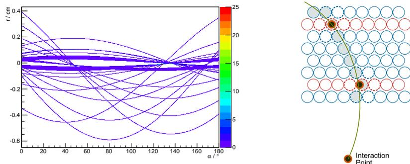
Figure 3: *Left*: Hough Transform of 68 hit points (STT, MVD).  $\alpha$  is evaluated every  $0.1^\circ$ . Thrust is used for computation, ROOT [4] for displaying, and CUSP [5] for providing fast, templated methods to interface between both using the GPU. *Right*: Sketch of Triplet generation of the Triplet Finder.
