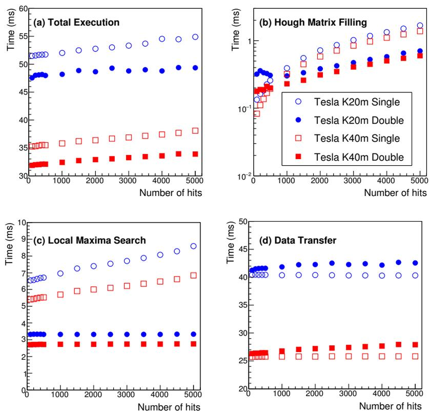
Figure 4: Execution timing as a function of the number of the hits for multi-GPU configuration. (a) Total execution time; (b)  $M_H$  filling timing; (c) local maxima search timing; (d) device-to-host transfer time.
