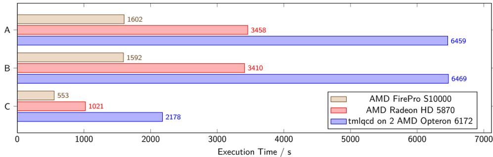
Figure 2: HMC performance for different Setups A, B and C (setup A having the smallest fermion mass) for  $N_\tau = 8, N_\sigma = 24$ . The HMC is compared on different GPUs and compared to a reference code [15] running on one LOEWE -CSC node.
