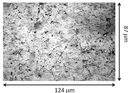
Figure 2: Nuclear emulsion image. High-energy tracks are orthogonal to plane.
