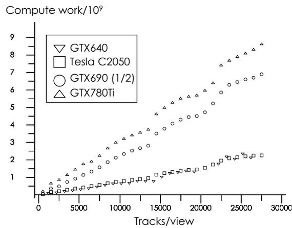
Figure 9: Compute work ( $\text{Cores} \times \text{Clock} \times \text{Time}$ , arbitrary units) for several boards. For GTX690, only one GPU is considered.
