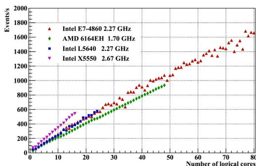
Figure 4: Scalability of the FLES package on many-core servers with 16, 24, 48 and 80 logical cores.
