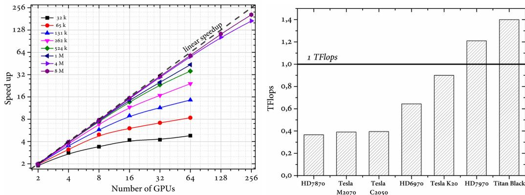
Figure 2: Left panel: speed up of the code `HiGPUs` as a function of the number of used GPUs for different  $N$ -body systems with  $3.2 \times 10^4 \lesssim N \lesssim 8 \times 10^6$ . The dashed line corresponds to the maximum computing efficiency (linear speedup). Right panel: performance (in TFlops) of `HiGPUs` running on single, different GPUs. For the scalability tests we used the IBM DataPlex DX360M3 Linux Infiniband Cluster provided by the Italian supercomputing consortium CINECA.
