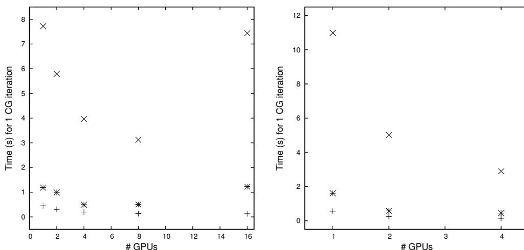
Figure 2: Strong scaling using lattice volume  $V = 32^4$  with, respectively, 1,2,4,8,16 Tesla GPUs (left plot) and 1,2,4 Kepler GPUs (right plot). The data correspond to the CG algorithm with preconditioning **i** (+), with preconditioning **iv** (x) and with preconditioning **iii** in single precision (\*).
