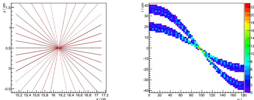
Figure 2: Schematic visualizations of Hough Transforms with coarse step sizes  $\alpha$  for illustration. *Left*: Different lines going through a hit point (center) are sampled in  $10^\circ$  steps with Equation 1. *Right*: Hough space for a set of STT hit points, the  $\alpha$  granularity is  $2^\circ$ .
