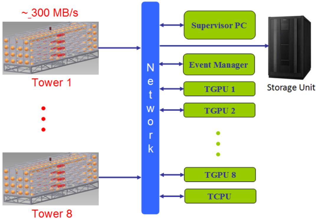
Figure 1: Proposed DAQ based on CPU-GPU structure.
