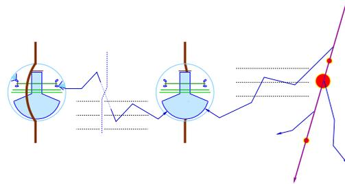
Figure 2: Typical simulation scenarios: photons emitted by the detector are tracked as part of the calibration procedure (left). Cherenkov photons emitted by a passing muon and cascades along its track are tracked to simulate the typical IceCube events (right).
