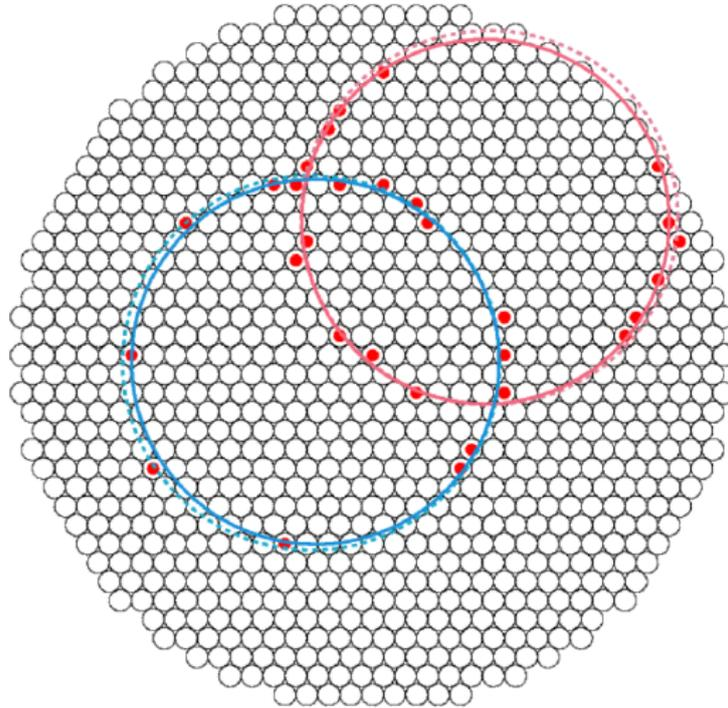
Figure 2: Two rings reconstructed by Almagest's algorithm (solid line). The dotted ring represent the real ring position. The small circles represent the PMTs positions within the NA62 RICH.
