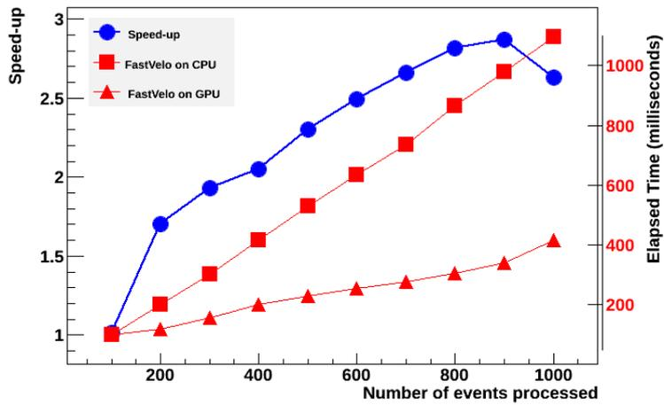
Figure 2: Tracking execution time and speedup versus number of events using a 2012 MC sample of  $B_s \rightarrow \phi\phi$  decays ( $\nu = 2.5$ ). The GPU is compared to a single CPU core (Intel(R) Core(TM) i7-3770 3.40 GHz).
