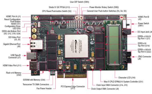
Figure 3: NaNet as a FPGA-based NIC implemented using an Altera development board (Stratix IVGX230 FPGA).
