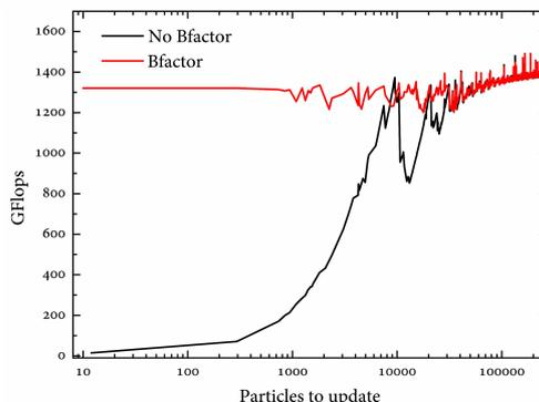
Figure 1: The effects of the **Bfactor** optimization on the performance of a GeForce GTX TITAN Black (measured in billions of floating point operations per second, GFlops) as a function of the number of particles that need to be updated (according to the block time steps distribution). The results were obtained using the  $N$ -body code HiGPUs with  $N \simeq 260,000$ .
