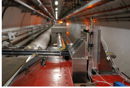
Fig. 8: ARM1 detector pre-installed in the TAN location in the LHC tunnel.
