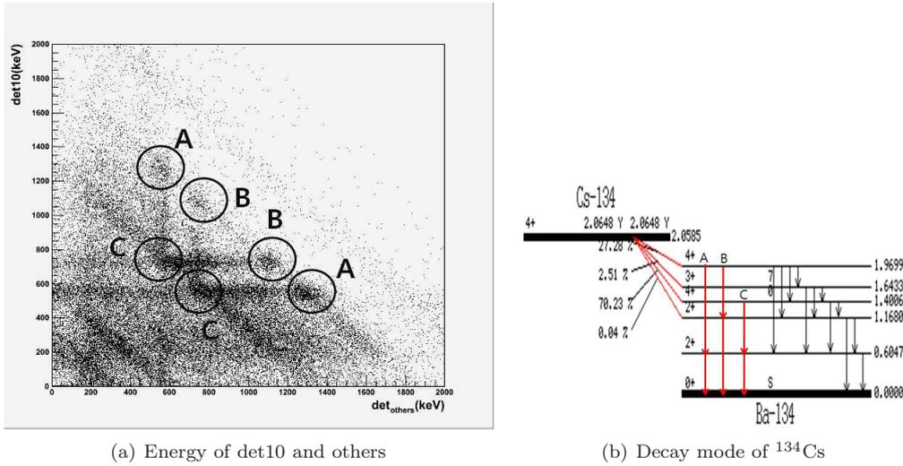
Figure 2: Identification of decay mode of  $^{134}\text{Cs}$  with detector arrays.
