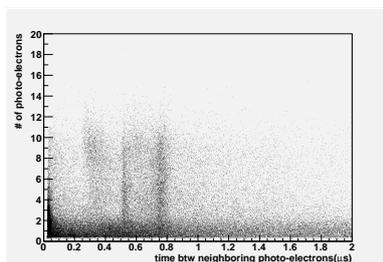
Figure 3: Signal size and time distribution of afterpulse.
