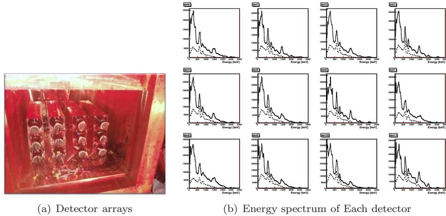
Figure 1: Detector arrays and their energy spectrum, at (b) dashed line represents multiple events.
