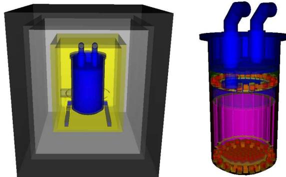
Figure 1: Left: The XENON100 detector inside its shield as it was simulated within the GEANT4 framework (the colors represent: two layers of lead - dark grey, polyethylene - light grey, and copper - yellow, water tanks are not shown; on the left side of the cryostat - lead brick for calibration with Am-Be source); Right: The closeup view of the detector (blue - stainless steel, magenta - PTFE, yellow - copper, orange - PMTs).
