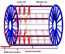
Figure 2: The laser calibration system.
