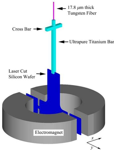
Figure 4: A diagram of the ALP pendulum.
