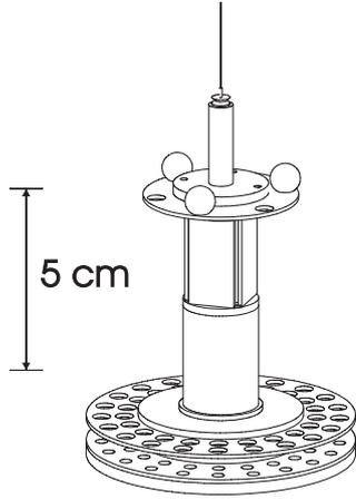
Figure 2: A scale drawing of the ISL pendulum.
