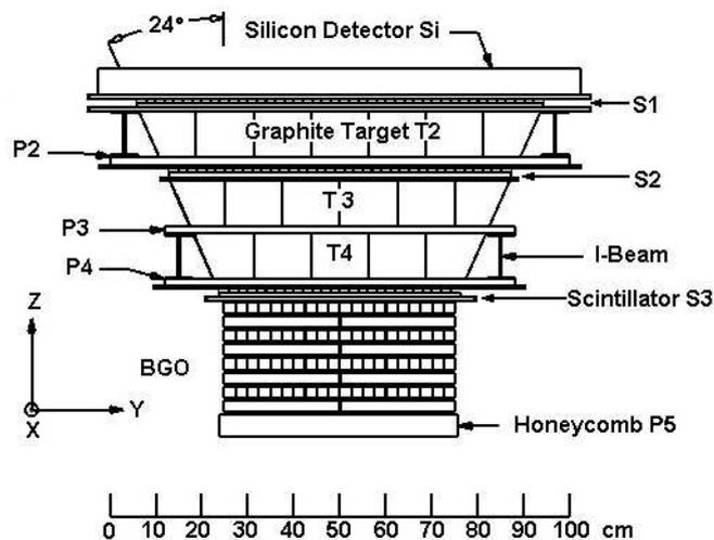
Figure 1: The ATIC detector. The top layer of silicon detectors is used to determine the magnitude of the incoming charge. Three layers of graphite, interspersed with scintillation hodoscopes for tracking, enhance the early interaction of incoming hadronic CRs. A Bismuth-Germanium-Oxide calorimeter with 18–22 radiation lengths depth is located at the bottom of the instrument.
