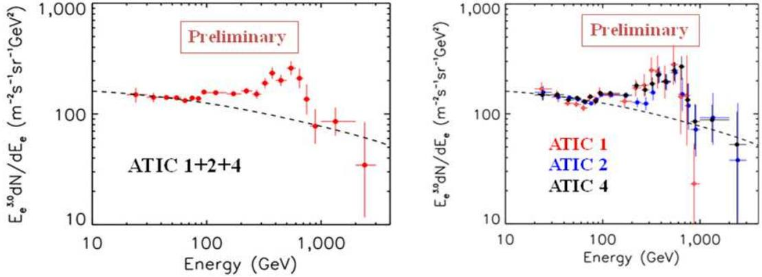
Figure 2: The total  $e^+ + e^-$  spectrum measured by ATIC. The first and second flight (ATIC 1 & 2) showed an enhancement of  $3.8\sigma$  centered around 600 GeV. The fourth flight (ATIC 4) showed the same feature with increased statistics resulting in an overall significance of  $5.1\sigma$ .
