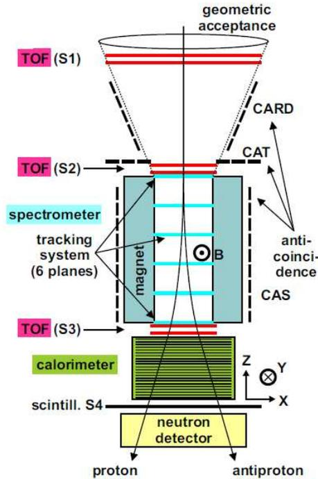
Figure 3: The PAMELA experiment. The magnetic spectrometer of this instrument is capable of determining the sign of the charge of detected particles to energies  $> 200$  GeV. PAMELA was launched in June 2007 onboard a Russian satellite and has taken data continually since launch.
