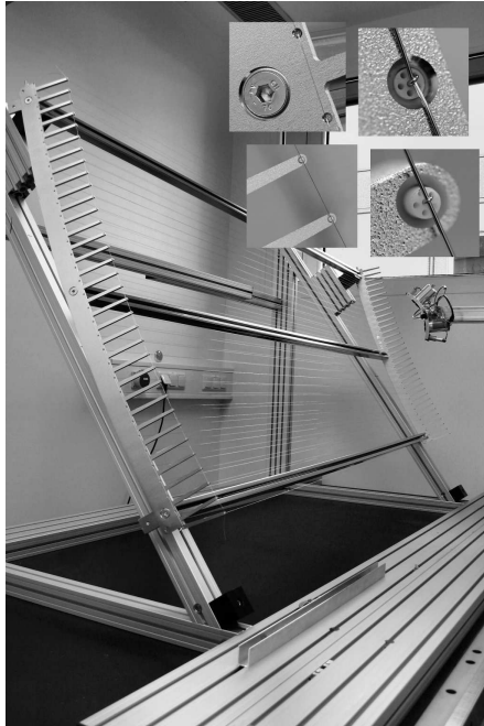
Figure 5: A double-layer wire electrode module on the 3-axis measurement table for quality assurance. The fixing of the wires inside the ceramics holders (see inserted smaller photos right) with the connecting wires is checked with a high-resolution camera, whereas wire position and wire tension are monitored by a specially developed 2-dim. laser sensor [26].
