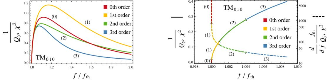
Figure 3: Plots of the 0th, 1st, 2nd and 3rd order approximations of  $1/Q_{\gamma'}$  (solid line) and its derivative (dashed line) against frequency / threshold frequency for the  $TM_{010}$  mode in a cylindrical cavity of unity aspect ratio ( $L = 2R$ ) with tuning performed by changing the size of the cavity whilst maintaining the aspect ratio.
