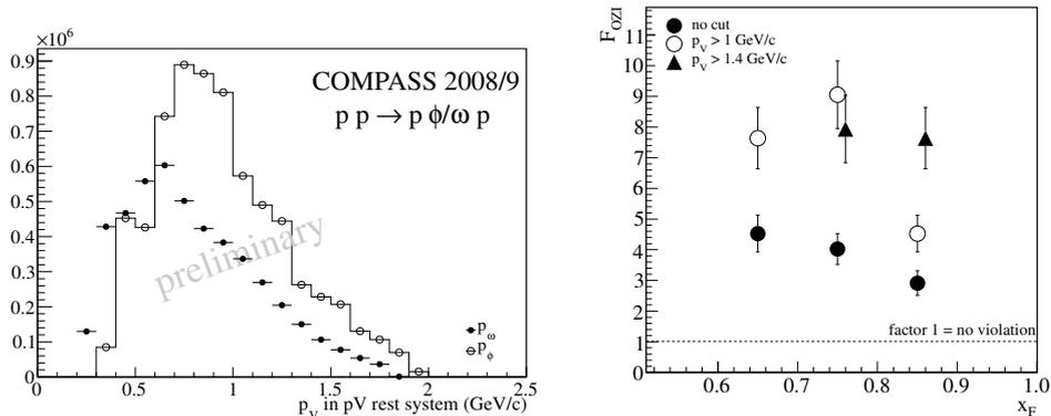
Figure 1: Left: The vector meson momentum  $p_V$  in the rest frame of the  $pV$  system, where  $V$  refers to  $\phi$  (white dots) or  $\omega$  (black dots). The  $\phi$  histogram has been scaled by a factor of 100. Right: OZI violation factor  $F_{OZI}$  as a function of  $x_F$  for different  $p_V$  cuts.
