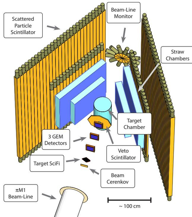
Figure 2: Schematic view of the planned detector setup for the MUSE experiment.
