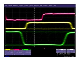
Figure 3: Deterministic latency of NaNet<sup>3</sup> SerDes: phase alignment of the transmitting (upper) and receiving (central) clocks.
