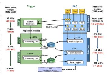
Figure 1: A scheme of the ATLAS trigger system; values in red are indicating the data-taking conditions during the first run of the LHC ('10-'12) while values in black represents the design conditions, expected to be reached during the upcoming run (starting in 2015).
