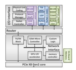
Figure 1: NaNet architecture schematic.
