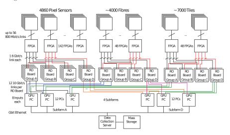
Figure 3: Readout scheme of the Mu3e detector design. [6]
