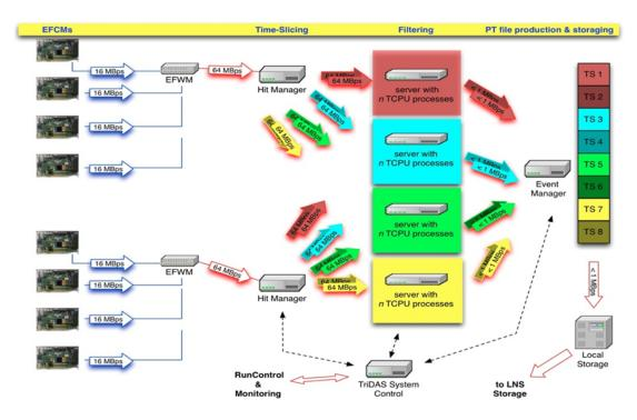
Figure 3: DAQ system for NEMO Phase II and the trigger scheme.
