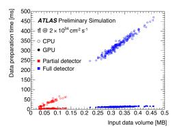
Figure 4: Bytestream decoding and clustering show a 26x speed-up on NVIDIA C2050 GPU vs single-threaded Intel E5620 CPU. [8]
