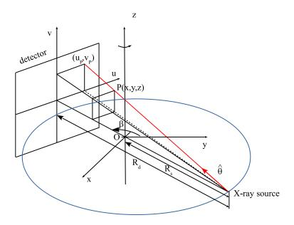
Figure 1: Cone-beam CT geometry.
