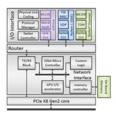
Figure 3: NaNet as a FPGA-based NIC implemented using an Altera development board (Stratix IVGX230 FPGA).
