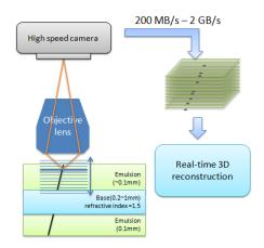
Figure 1: Schematic of scanning microscopes
