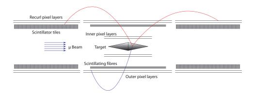
Figure 2: Schematic of the Mu3e detector design.
