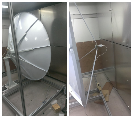
Figure 3: The setup for the search in K_u band. The parabolic dish designed for CS broadcast reception faces on the plane reflector made up of four aluminum plates.
