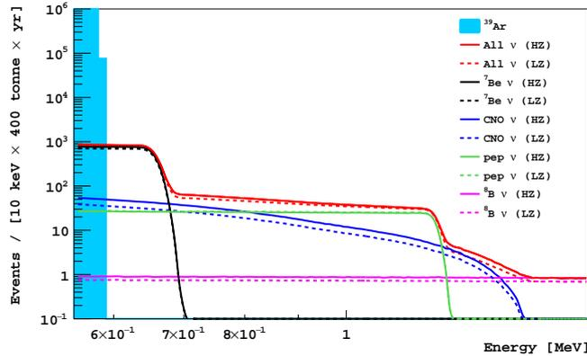
Figure 1: Simulated solar neutrino spectra in a 400 tonne-yr LAr TPC exposure, assuming  $\sigma = 1.3\%$  energy resolution at 1 MeV, corresponding to a PE yield of 6 PE/keV. The blue shaded area represents the tail of the  $^{39}\text{Ar}$  contamination, intrinsic to underground LAr.
