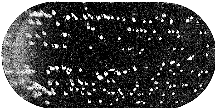
Fig. 9b \Delta t = 10 ms, R \sim 0.45 mm, b \sim 4 bubbles/cm
