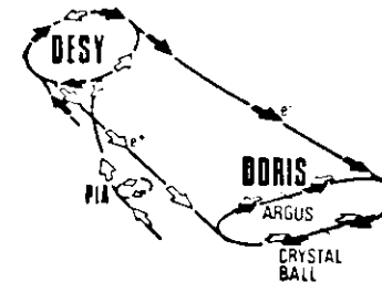
Figure 3. DORIS II with its injection system (DESY and PIA) and its experiments Crystal Ball and ARGUS
