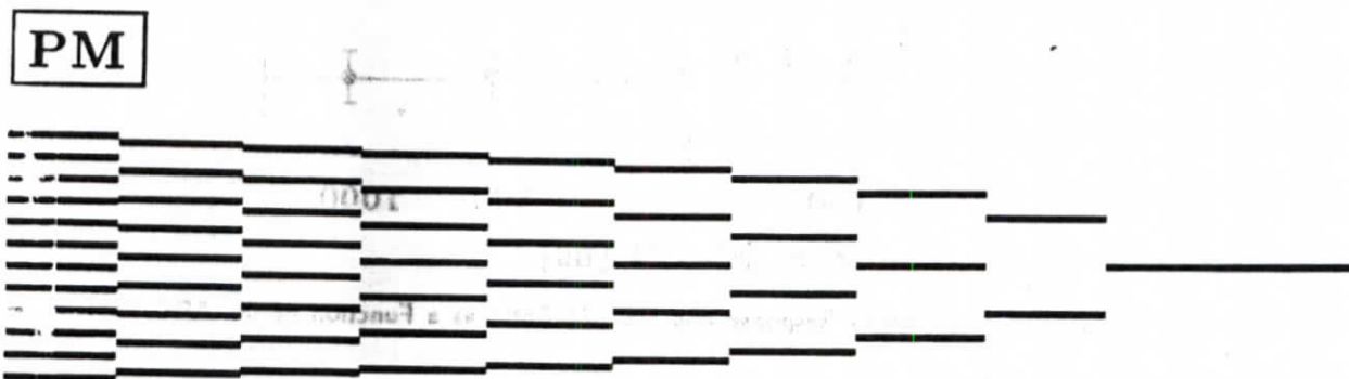
Figure 5.27: Pattern of a Graded Light Filter used to improve the Longitudinal Nonuniformity of the Wavelength Shifter Bars in the T60B2 Calorimeter (PM: Photomultiplier Side)
