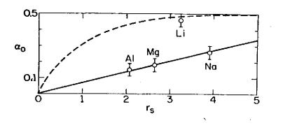
Fig. 2. Exponents  $\alpha_0 \xrightarrow{vs.} r_s$ . Solid line:data; dashed line: theory. The exponent for Li is obtained from K edge data. (Ref.4,10).
