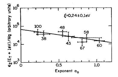
Fig. 1.  $\ln \epsilon_2 \underline{vs}$ .  $\alpha_0$  for  $Mg_xSb_{1-x}$ . The values of x are denoted on the figure. A negative slope indicates  $\xi < 1eV$ . (Ref.4).
