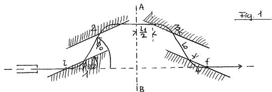
Let the fields be separated by field free lengths  $L_o$ ,  $L_1$ . The figure shows the path of a particle of the principal energy, say "W<sub>p</sub> = 40 MeV, which enters the magnetic field under the angle  $\emptyset$  o/2 between particle direction and field limit. This particle is bent by field 1 through the angle  $\emptyset_o$ ,
