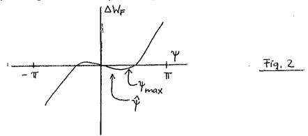
The maximum final energy deviation may be calculated from equ. (9). By differentiating (9) with respect to  $\Upsilon$  one finds the angle  $\widehat{\Upsilon}$  at which the maximum occurs, giving the final maximum deviation
